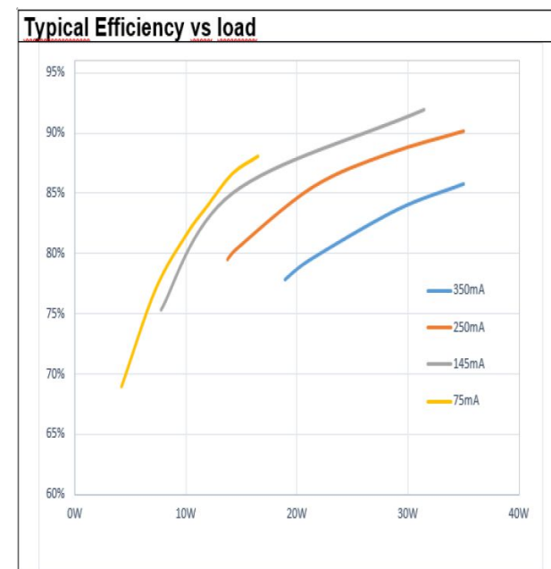
OT FIT 35/220-240/350 D LT2 L Typical Efficiency vs. Load (230 V / 50 Hz)
